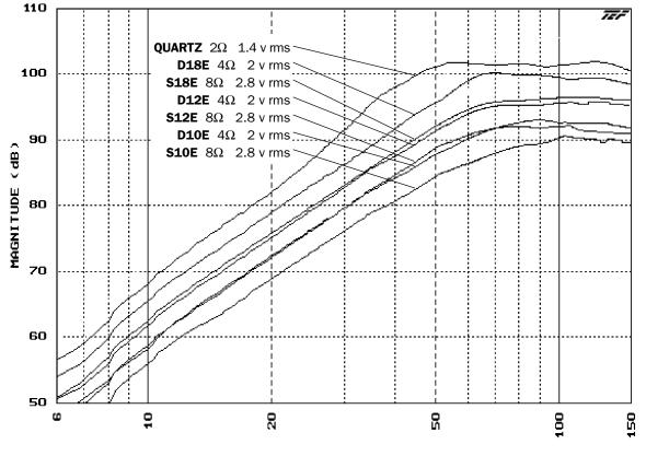
The measurement was made on a Techron TEF20 analvzer with SoundLab TDS software. The test signal is a 15 second swept sine wave. The microphone is a Bruel & Kaer 4007 and was placed on the woofer axis at 1 meter from the baffle. The measurement has a 2 Hz resolution and there is no smoothing applied to the display.
