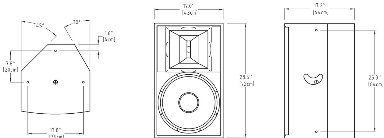
⊕ = Center of Gravity ○ = M10 Threaded Rigging Point
