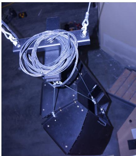
True Time-Alignment™ requires much more than just physically lining up the loudspeaker components. It requires consideration of the driver placement, driver delay and adjustment of the crossover delay parameters. This achieves the precise simultaneous acoustical arrival time of each driver throughout the crossover region.
