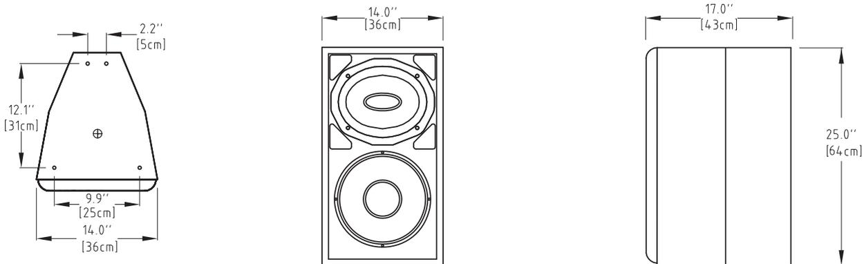
⊕ = Center of Gravity      ○ = 5/16"- 18 Threaded Rigging Point
