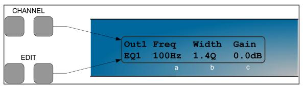
Pressing the edit navigation buttons gives access to the various pages of parameters available for each channel. The currently selected page is shown in the bottom left hand corner of the display, this is omitted on some pages where the function is obvious. The screen shows up to three (normally related) parameters for a given part of the processing functions on a given channel.
