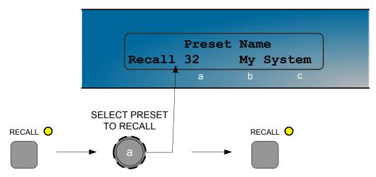
Users can develop their own Preset based on one of the Basic or Factory Presets stored within the device. Once a basic or user Preset has been recalled, a user has complete freedom to adjust any or all of the parameters. Factory Presets can be used as the basis for user Presets but they have some parameters that are predefined as a function of the loudspeaker system. These parameters are 'hidden' from the user, as they should be constant regardless of application.
