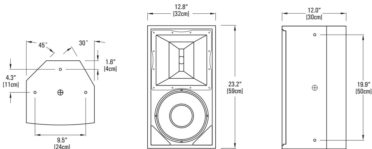
⊕ = Center of Gravity   ○ = M10 Threaded Rigging Point
