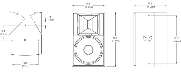
$\bigoplus$  = Center of Gravity  $\circ$  = M10 Threaded Rigging Point
