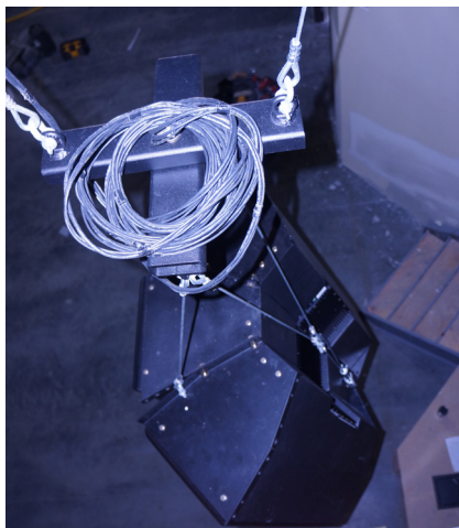
The Crystal2 is shown in an array using the Crystal rigging pan
