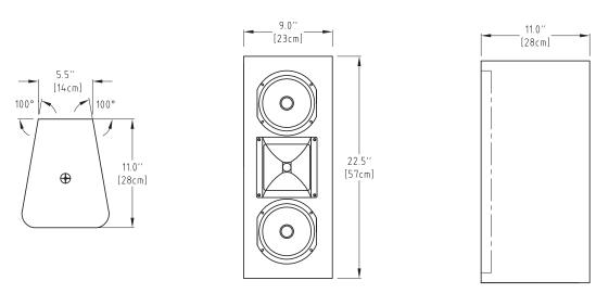
$\oplus$  = Center of Gravity  $\circ$  = 5/16" -18 Threaded Rigging Point
